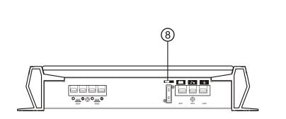
Off to a normal operating range. If activated by an overload condition, the source of the overload must be found and corrected to resume operation of the amplifier. Most overload conditions are caused by mis-wiring or operation into incorrect speaker loads. Re-check all wiring and connections if this situation occurs and correct as necessary.
